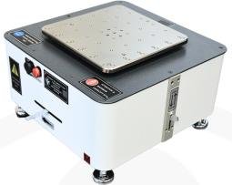
K-KAM Mass properties Measurement Systems are products with advanced features that can measure both the center of gravity and inertia moments of objects of various weights without size limitation.
